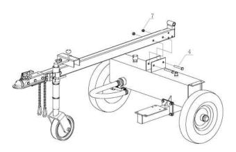
Fix the support leg (#31) to the tow bar by a pin (#29),Bolt M10X75(#30),Lock Nut M10(#22) and R Pin(#16).
